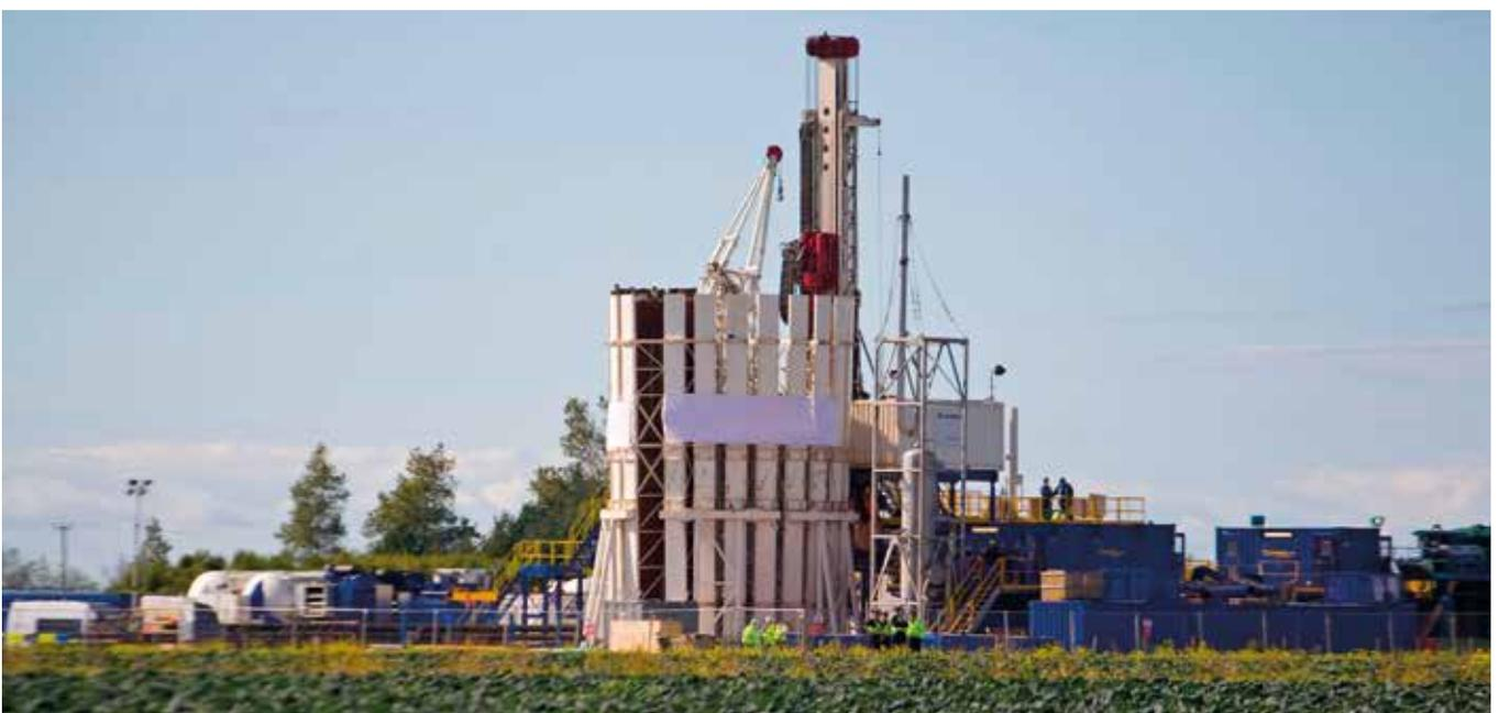
Drilling equipment at a shale gas drill site, Southport.
